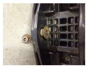
2. Remove stock ski rubber. Trim the nubs or ridges off with a tin snips, wire cutter, knife etc so it can sit down farther in the ski saddle.
