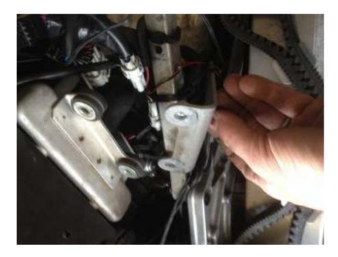
6. Slide the fan shroud into position as shown. Slide the clutch side in behind throttle cable first. Once in place, bolt it fast using the (4) nylon spacers and counter sunk screws. The spacers go between the shroud and radiator.
