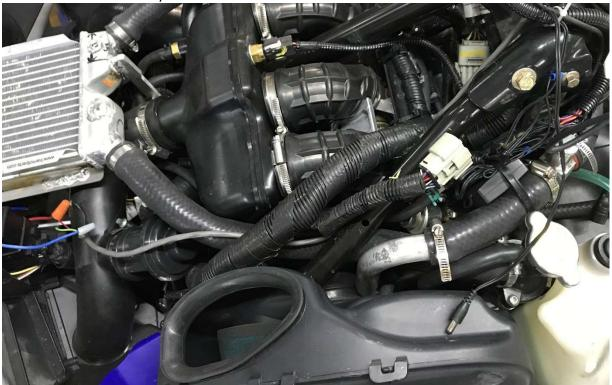
11. Using the 6" long hose connect the T fitting to the aluminum coolant elbow as shown below.
