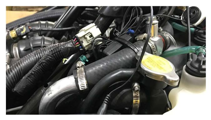
12. Route the 27" long hose as shown in the photo below and connect it to the T fitting and the throttle side nipple of radiator. If there are any kinks in hose shorten hose as needed.
