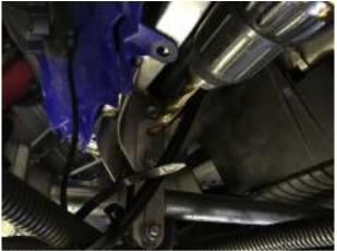
9. Install the collar between the steering hoop plates and bolt it in place with the M8 bolt and lock nut.
