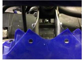
10. Sit on sled and see how the relocate feels if it feels too far forward you can flip the plates around as shown so the relocate isn't as far forward.
