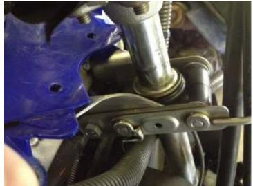
11. Re-route cables and wire looms as shown below. Be sure to re-route throttle cable so it remains under the handlebars and does not cross over the bar. If throttle cable is not re-routed could be under tension in a full right hand turn. The wire loop on the stud plate is no longer used and can be cut off if desired.
