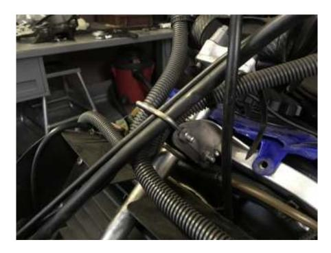
3. Proceed to unbolt the steering post from the steering hoop. There are two 12mm nuts. The bolt studs are attached to plate with the wire loop. Bend the loop a bit so the wires & cables can be undone to allow the stud bracket to slide out.
