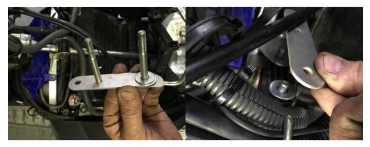
7. Install washer plate with tangs and nuts on upper steering block and tighten.
