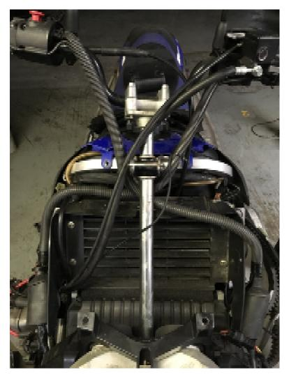
12. If you opted for the farther forward positioning, trim the dash panel accordingly so it clears the relocated steering post.
