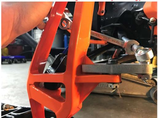
10. Tighten tie rod ball joint to the MPS arm and install the cotter pin.
