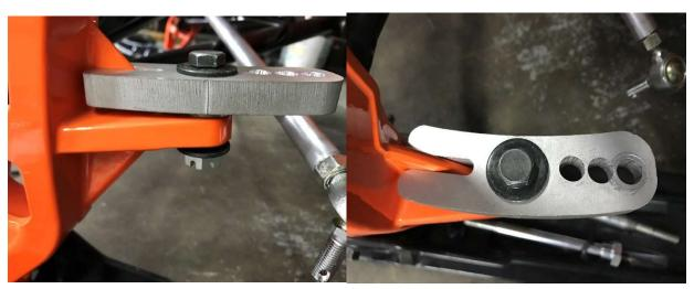
3. Remove the push pins so the rubber boot can be pulled away to gain access to the inner tie rod connection. Loosen the jam nut and remove the stock tie rod.
