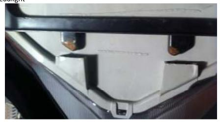
3. When headlight is seated properly in the mounting frame use a sharple marker to trace a partial circle around each isolator.
