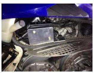
8. Reconnect the fan using the jumper harness supplied and then proceed to install hood and side panel.
