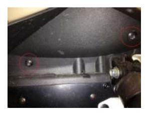
4. Remove the fuse box from the bracket that's attached to the coolant reservoir so the bracket can be unbolted from the coolant reservoir. Once the bracket is removed the reservoir can be re-attached.
