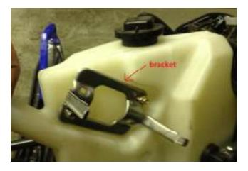
5. Using the two factory bolts and (2) nuts supplied attach the fuse box bracket to the BOP relocate plate.
